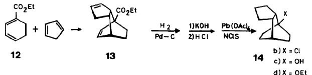
tricyclo[5.2.2.0<sup>2,6</sup>]undecane  $\underline{14b}$ <sup>[8]</sup>, synthesized from the cycloadduct  $\underline{13}$  of ethyl 1-cyclohexa-1,3-diencarboxylate ( $\underline{12}$ ) by catalytic hydrogenation, ester hydrolysis and lead tetraacetate decarboxylation in the presence of N-chlorosuccinimide (44 % overall yield).  $\underline{14b}$  solvolyzes about 95 times faster than  $\underline{1b}$  (see table 1).
